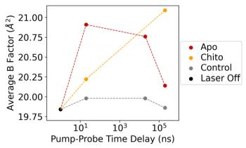
**Extended Data Fig. 4 | Effect of T-jump on average B-factor of refined apo and chitobiose-bound structures.** Models were refined against Laser Off, Experiment (apo or chitobiose bound), or Control structure factors. Controls exhibit similar B-factors across all time points, while B-factors for experimental
