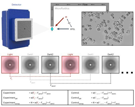
**Fig. 1** | **Schematic of T-jump TRX experiment.** Lysozyme crystals were delivered to the pump-probe interaction region via a microfluidic jet. Light and dark images were collected in an interleaved manner, with light images defined as those where the crystal was pumped with an IR laser at a defined time delay (Δt) before being probed by the XFEL. Dark images were collected with the IR
