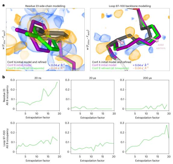
**Fig. 4** | **Explicit modelling of time-resolved structural changes. a**, For all pump-probe time delays, difference electron density maps were visualized at an absolute contour level of  $\pm 0.04 \text{ e}^- \text{Å}^{-3}$  alongside the refined models. Alternate conformations were manually modelled into the experimental difference density for several regions, including residues 23 and 97–100, then refined against ESFMs. An ANM was developed on the basis of the ground state (conformation
